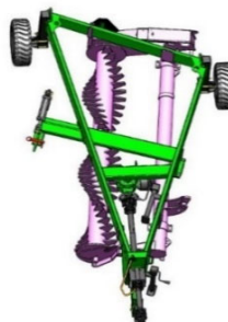
Shipping kit installed ready for truck
