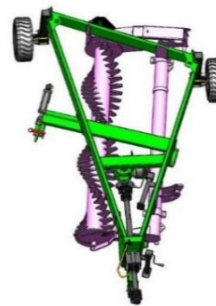
Shipping kit installed ready for truck
